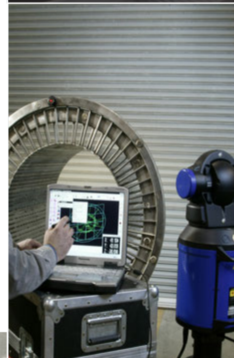
Laser Tracker Inspection
