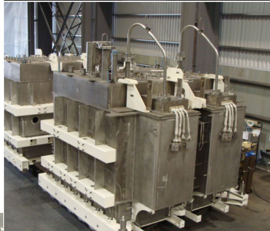
HLW Melter- Bechtel National
